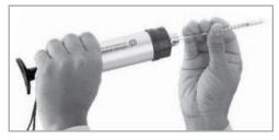
• Pull the handle at full stroke and wait for completion of sampling. Pull out the detector tube from the pump inlet and take the reading at the demarcation line between stained and unstained region.
