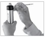
• Insert one end of the tube securely in the sampling pump inlet ensuring that the arrow on the detector tube points towards the pump. Align the guide marks (red dots) on the shaft and the stopper of the pump.
